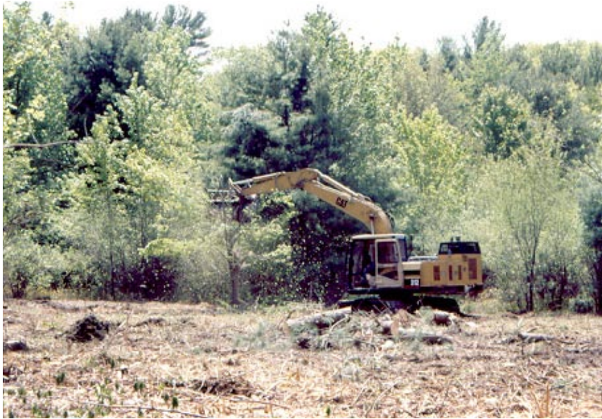
Figure 2. A Brontosaurus grinding or “mowing” a tree. All that remains of mowed trees are small strips of wood fiber on the ground. Photos by Matt Tarr.
