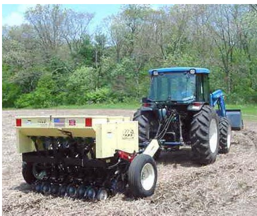
Figure 6. A no-till drill, such as a Truax® (pictured) or Great Plains® seeder, is the most effective means to plant fluffy warm-season grass seed. Photo by Paul Rothbart.
